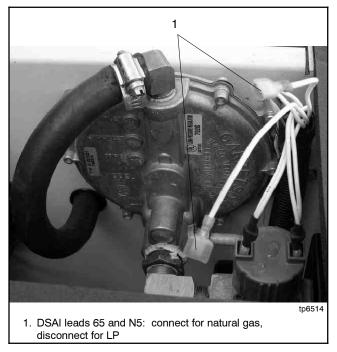
Figure 1-18 Digital Spark Advance (DSAI) Leads (located in generator set air intake area)
